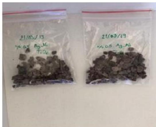
**Figure 4.** Ag-Ni TiO<sub>2</sub> coated volcanic stones
