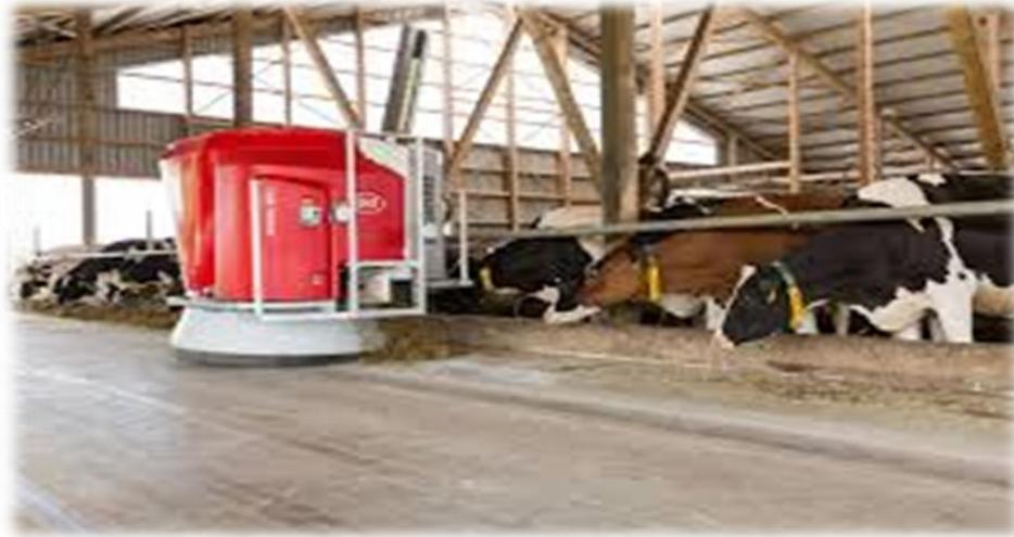
**Figure 2.** Feed Distribution In Robotic Systems (Anonymous 2019 h)
