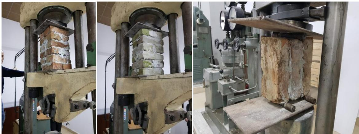
**Figure 6.** Prism masonry test and triplet shear test
