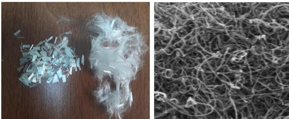
**Figure 1.** Synthetic fibers in a bundle and randomly distributed form (at left) SEM micrograph image of CNT (at right)
