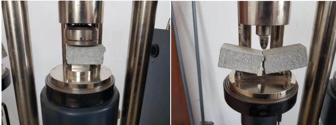
**Figure 5.** Mortar samples compression and tensile flexural test
