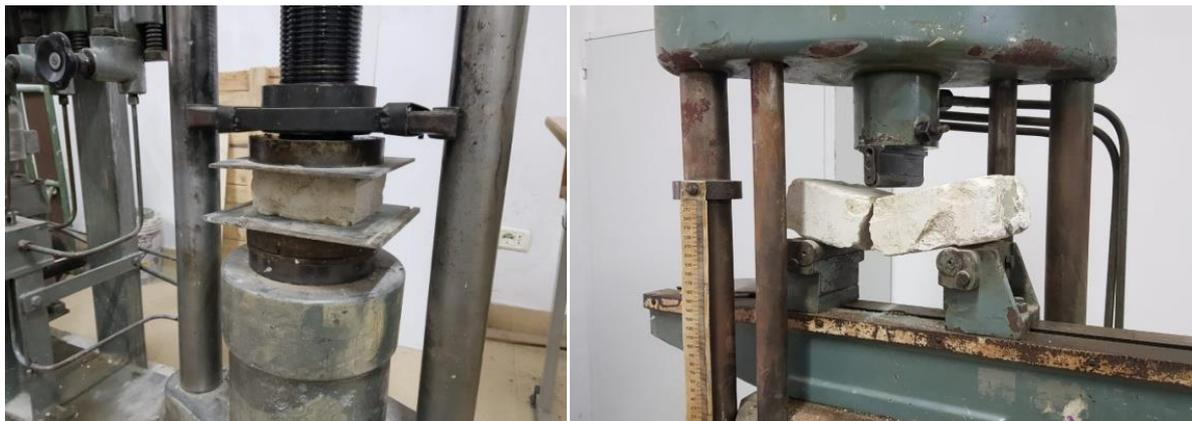
**Figure 4.** Brick compression and tensile flexural test
