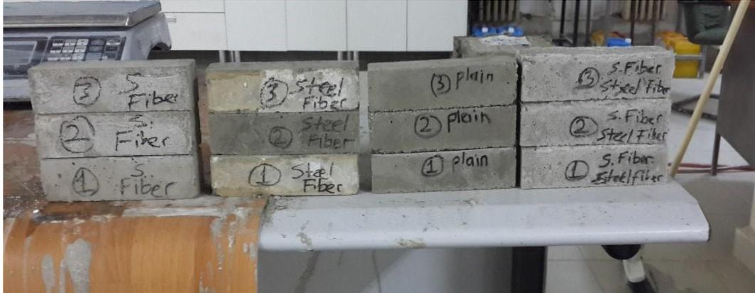
**Figure 2.** Specimens produced from four mixtures
