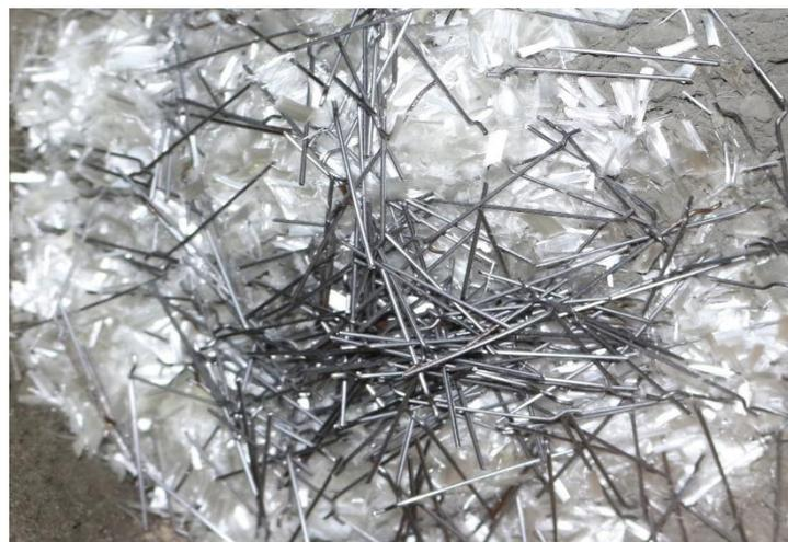
**Figure 1.** Polymeric and steel fibers
