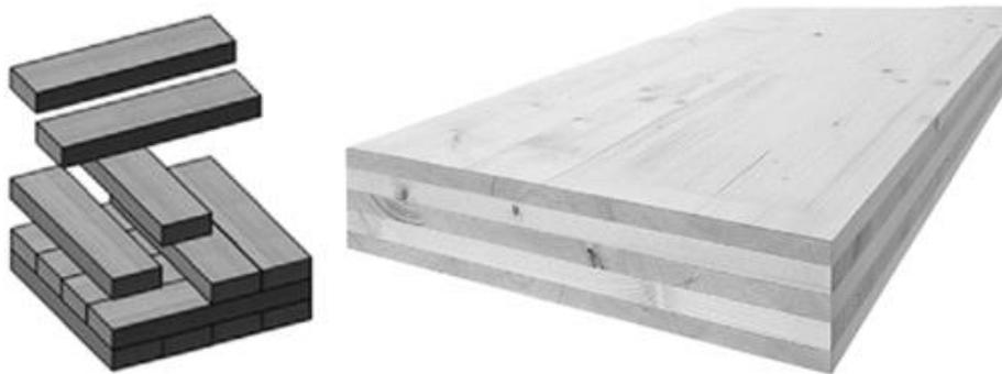
**Figure 1.** CLT concept and CLT panel (Pei, 2013)
