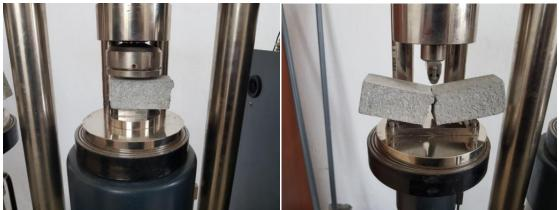
Figure 5. Mortar samples compression and tensile flexuaral test
