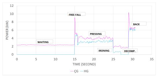
Figure 6 Power consumption graph for variable speed control
