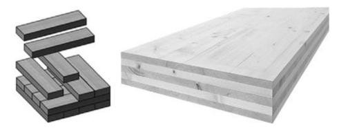
Figure 1. CLT concept and CLT panel (Pei, 2013)
