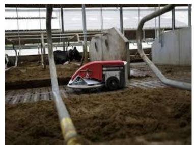
Figure 3. Manure Removal Robot in Robotic System (Anonymous 2019 1)
