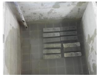
Figure 3. Thermostat controlled curing of specimens at 20±2 C
