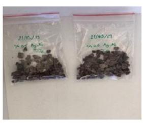
Figure 4. Ag-Ni TiO2 coated volcanic stones
