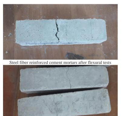
Hybrid fiber reinforced cement mortars after flexural tests Figure 6. Different cracks widths of specimens after tests
