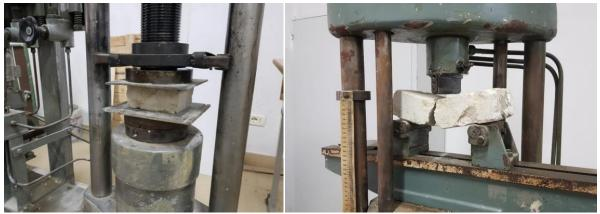
Figure 4. Brick compression and tensile flexuaral test
