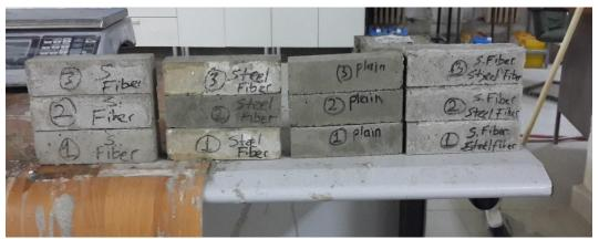
Figure 2. Specimens produced from four mixtures
