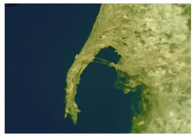
Figure 7. Flocculation of polymeric fibers in mortars
