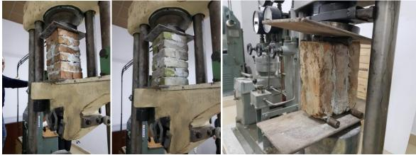
Figure 6. Prism masonry test and tripet shear test
