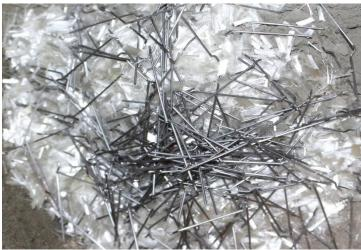
Figure 1. Polymeric and steel fibers
