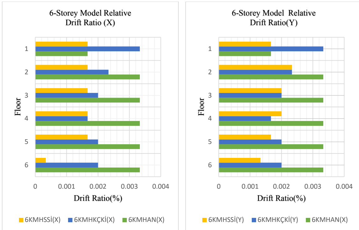
Figure 5. Comparison of relative drift ratio(%) of 6-storey hospital buildings in two different directions (X, Y)
