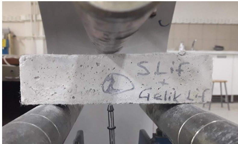
Figure 4. 3-point bending tests of hybrid fiber reinforced cement mortars
