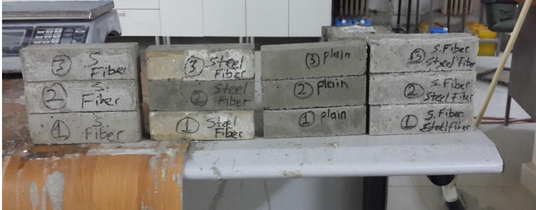
Figure 2. Specimens produced from four mixtures
