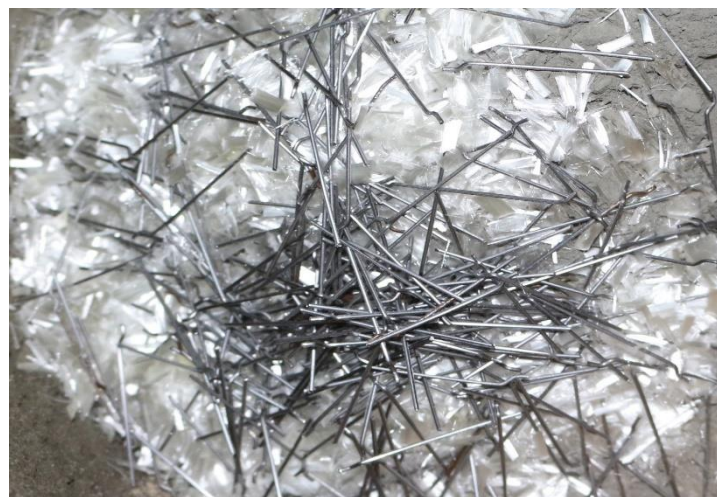
Figure 1. Polymeric and steel fibers
