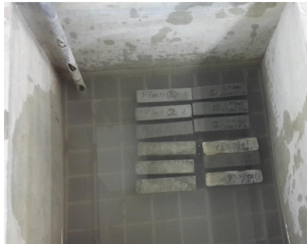
Figure 3. Thermostat controlled curing of specimens at 20\pm 2 C
