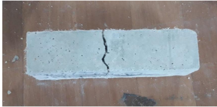
Steel fiber reinforced cement mortars after flexural tests
