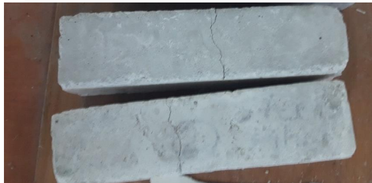
Hybrid fiber reinforced cement mortars after flexural tests
