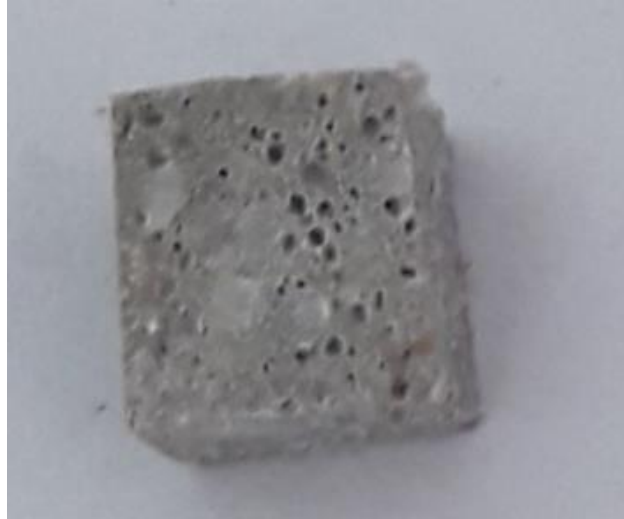
Figure 8. Entrapped air voids due to the inclusion of polymeric fibers
