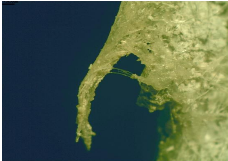
Figure 7. Flocculation of polymeric fibers in mortars
