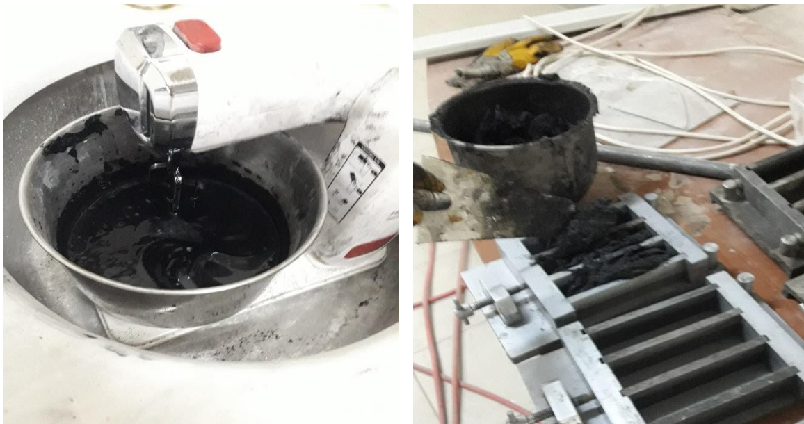
Figure 2. Preparing CNT solution (at left) and CNT incorporated cement mortars (at right)
