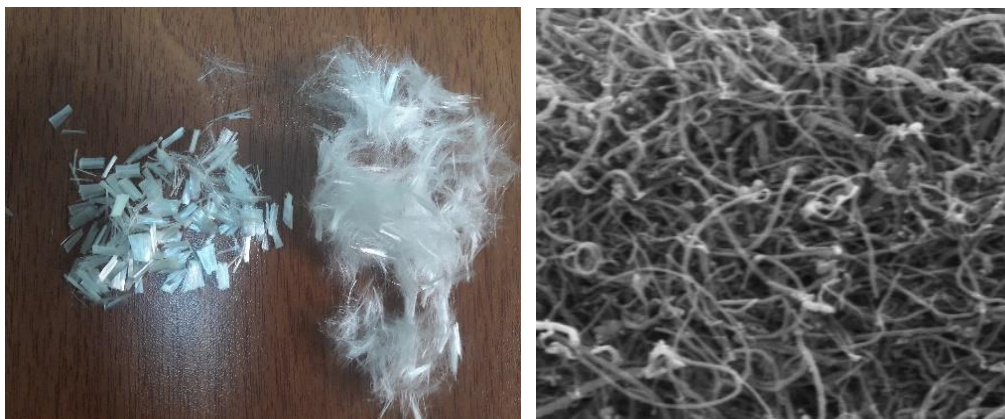
Figure 1. Synthetic fibers in a bundle and randomly distributed form (at left) SEM micrograph image of CNT (at right)
