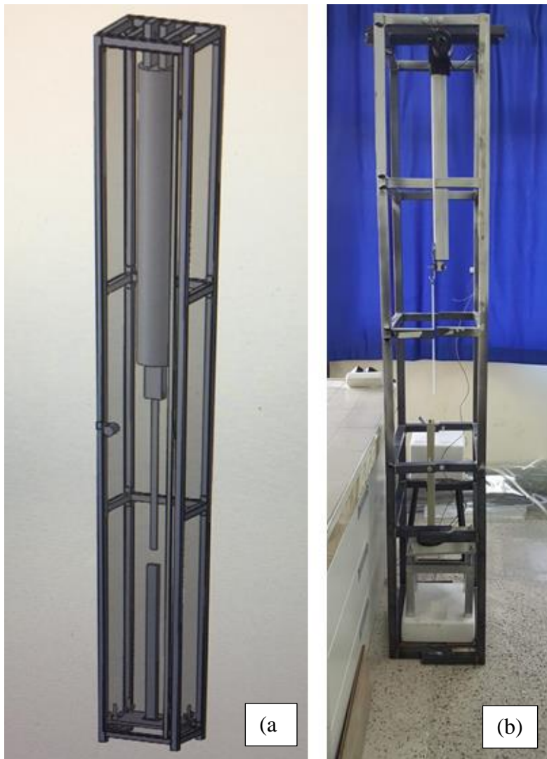
Figure 6. (a) AutoCAD drawing of dip coater and (b) the picture of final device
