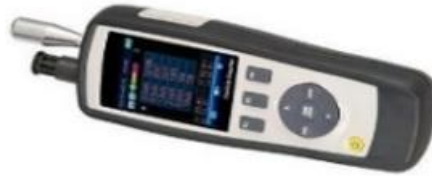
Figure 1. PCE – PC01 Particle Counter instrument for measurement of Particle matter
