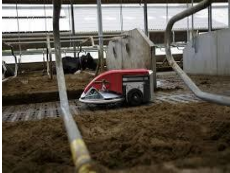
Figure 3. Manure Removal Robot in Robotic System (Anonymous 2019 1)
