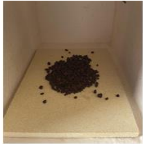
Figure 2. Drying of volcanic stones in ash oven
