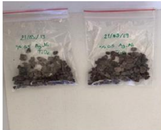
Figure 4. Ag-Ni TiO 2 coated volcanic stones
