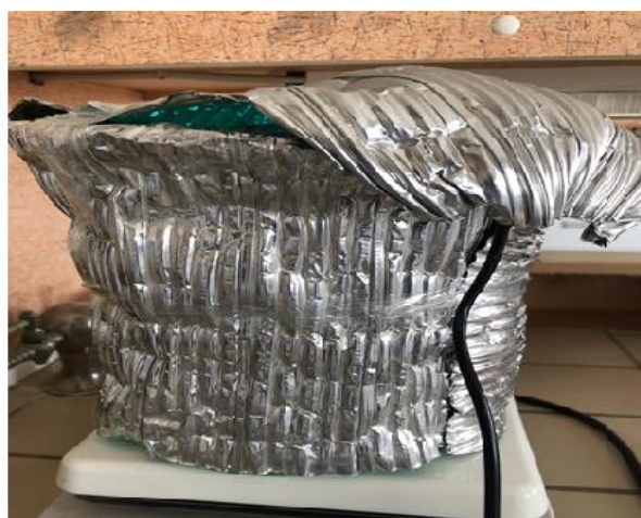
Figure 7. Mixing in batch reactor with UV light
