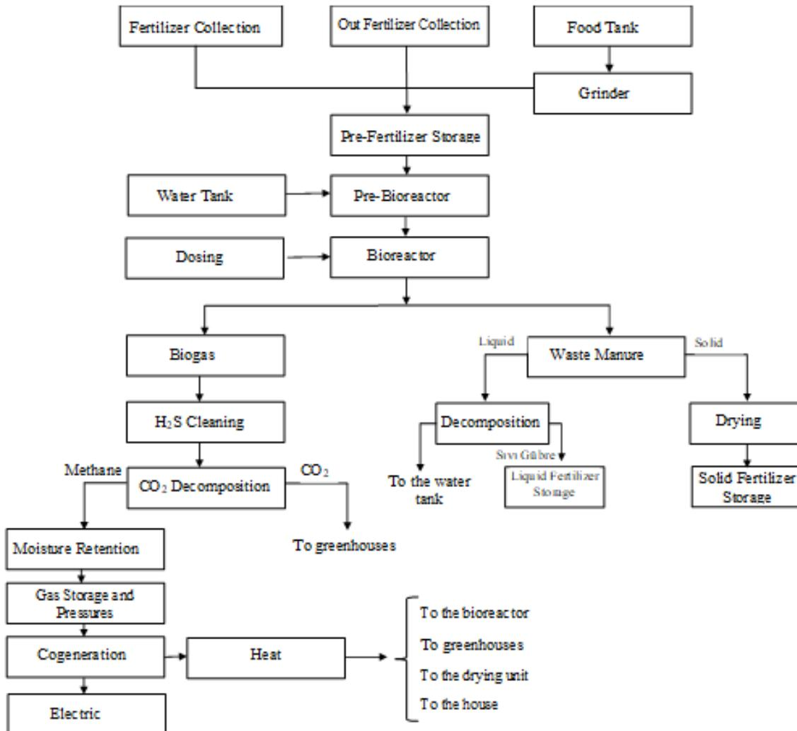
**Figure 3.** Work Flow Chart of the facility
