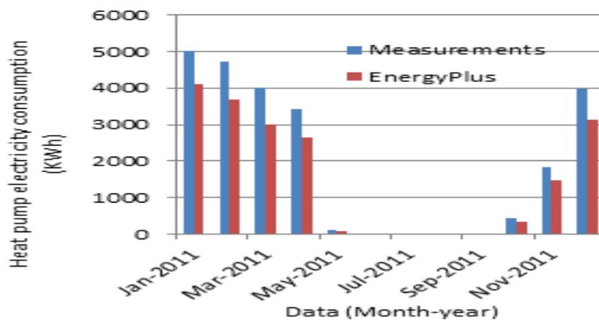
**Fig. 4.** Monthly comparison of electricity consumption between manual (Measurement) and automatic (EnergyPlus) control of the heat pump
