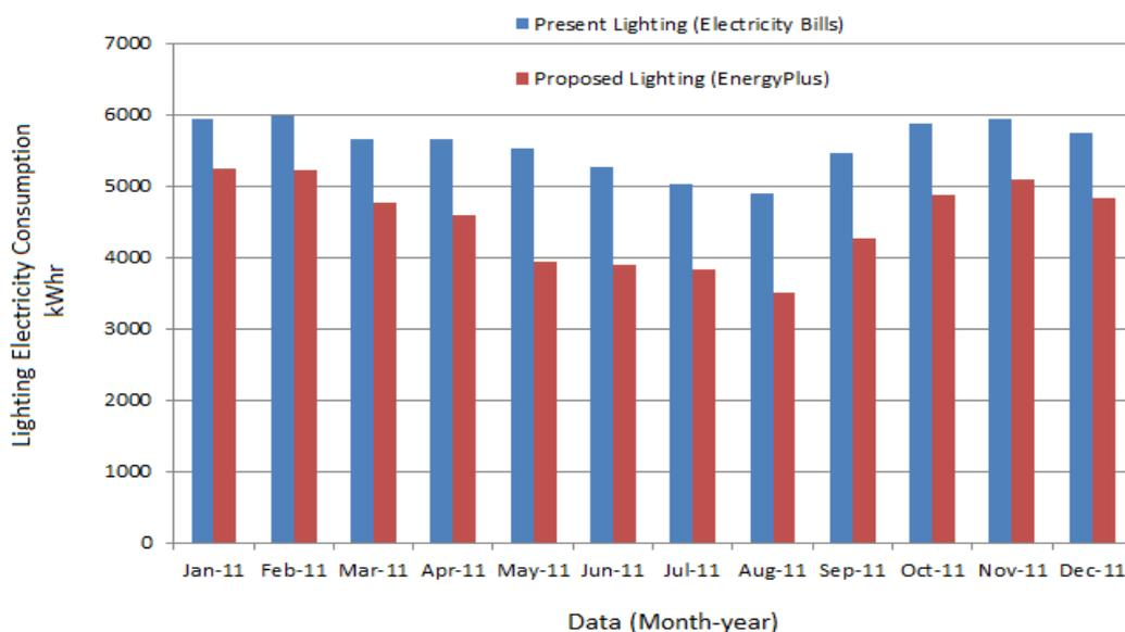
**Fig. 5.** Monthly present lighting v proposed lighting electricity consumption
