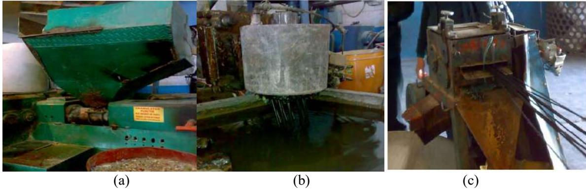
**Figure 7.** (a) Granulation (b) Pass the material through the fillers (c) Pass the material through the water bath into the cutter until the granules are obtained.
