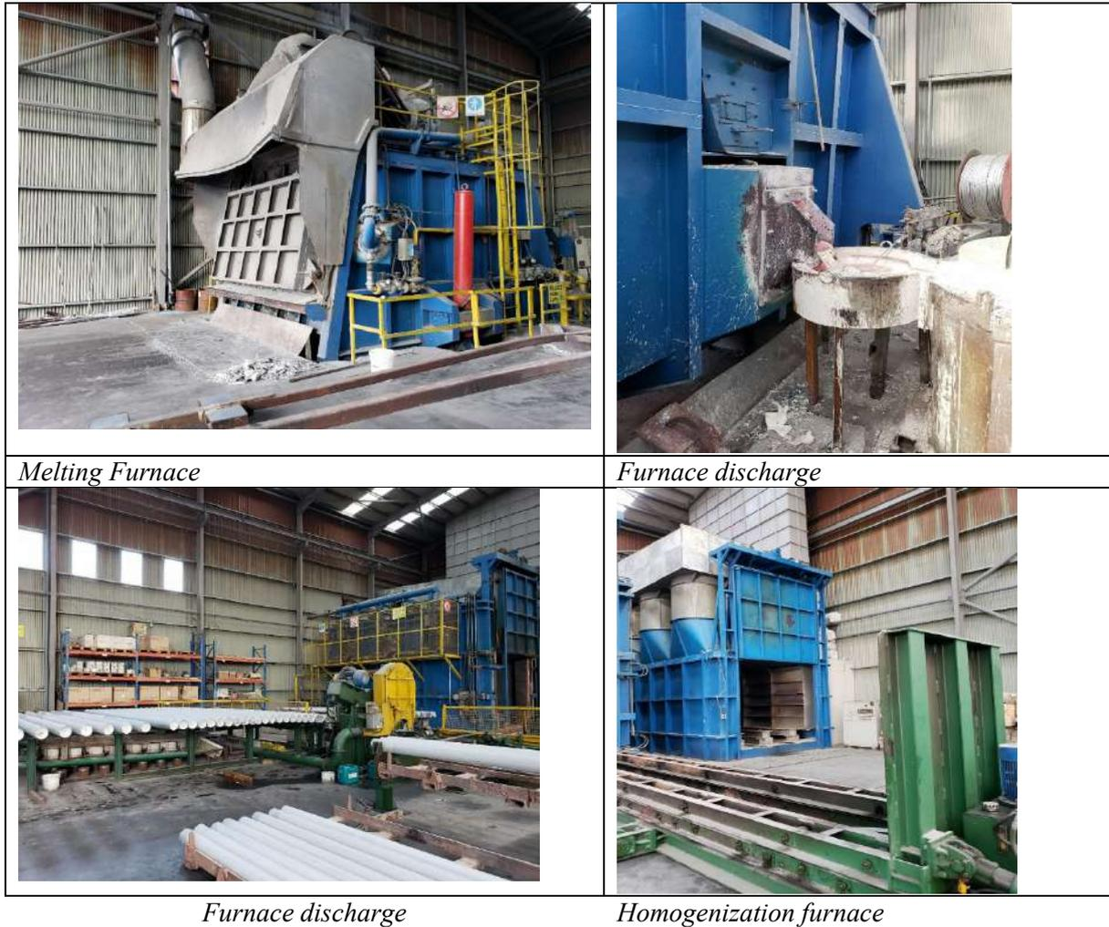
**Figure 5:** Aluminium Recycling equipments technology in Everest industry in Albania
