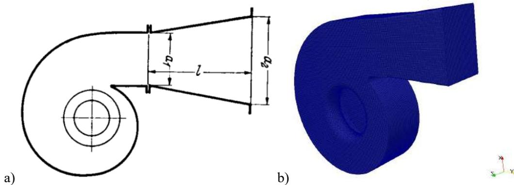
Figure 1. a) Improving the spiral casing by adding diffuser to the end (Eck 1973) [2]
