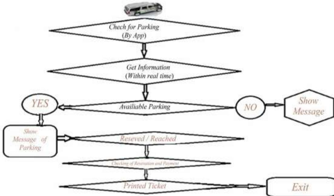
Figure 3. Flow chart of the process of the intelligent parking system
